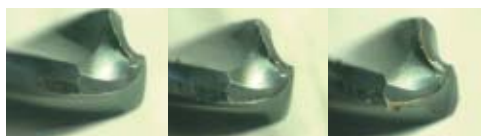
200穴 1000穴 2000穴 200 holes processing 1000 holes processing 2000 holes processing
