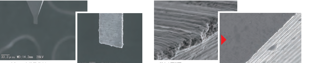
φ10μm 1枚刃 E/M 1 Flute End Mill
